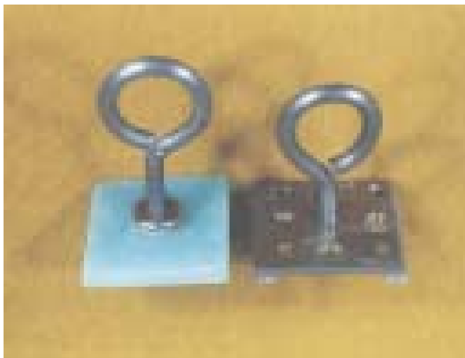
Fig 1: Metal nut with retentive threads embedded in the acrylic resin plate opposite to the test surface to which eye-bolt is screwed, (left); machined perforated metal impression holder with stops at four corners to which eye-bolt is screwed, (right).
