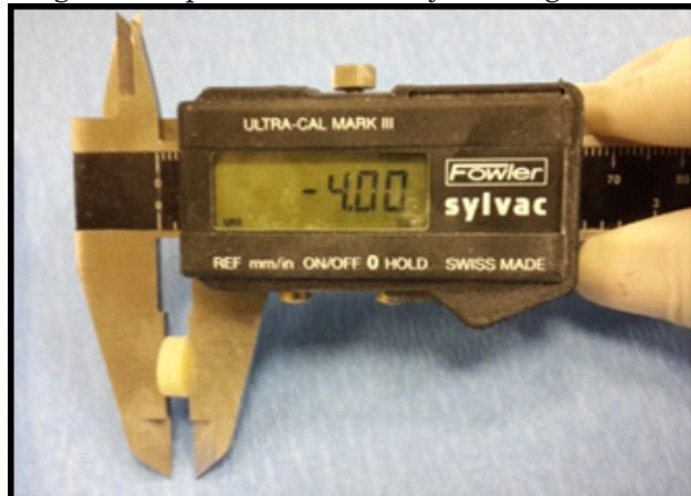
Fig 3: The verification of the samples' thickness using the micrometer
