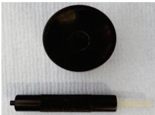
Fig 7: Funnel for loading the sample in the rotor along with the packing tool
