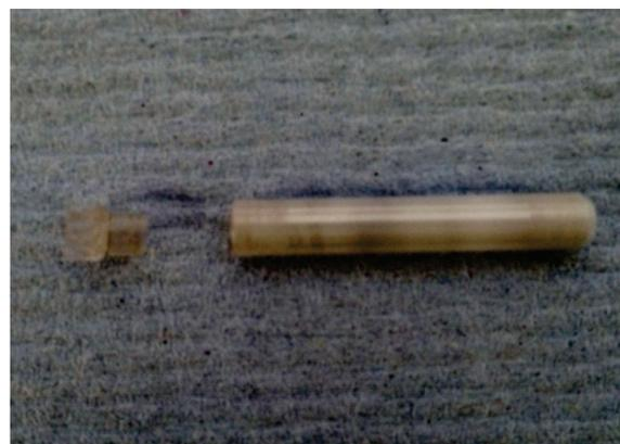
Fig 4: Rotor for packing the specimen
