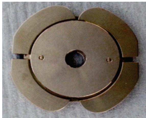
Fig 6: Tools for opening the caps of the rotor
