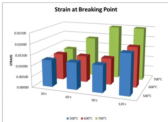
Fig. 1: Maximum strain at breaking point in relation to increasing Temperature (in degree centigrates) and Time (in seconds)
