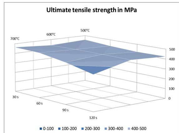
Fig.2: Ultimate Tensile Strength in MPa in relation to increasing Temperature (in degree centigrates) and Time (in seconds).
