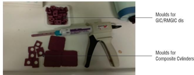
Fig 2: PVS Sheets, disc moulds, cylinder moulds in petri dish, gun
