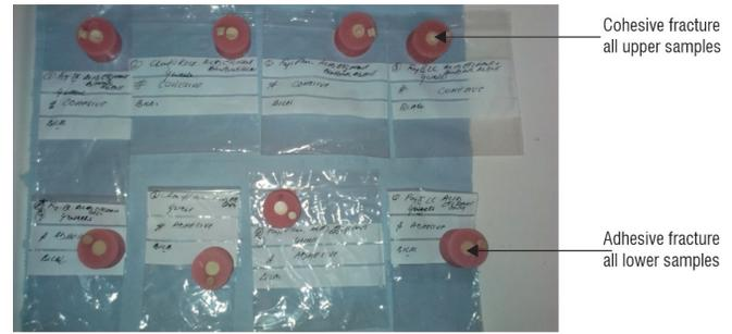
Fig 6: Samples containing Cohesive & Adhesive fracture
