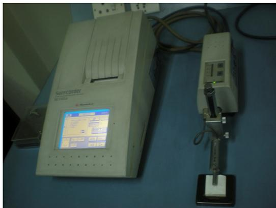
Fig 2: Profilometer used to assess enamel surface roughness parameters
