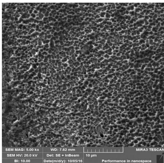
Fig 8: High magnification image of peripheral region of a Group B file showing dimples
