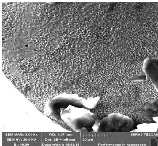
Fig 7: Peripheral region of a Group B file having a dimpled appearance
