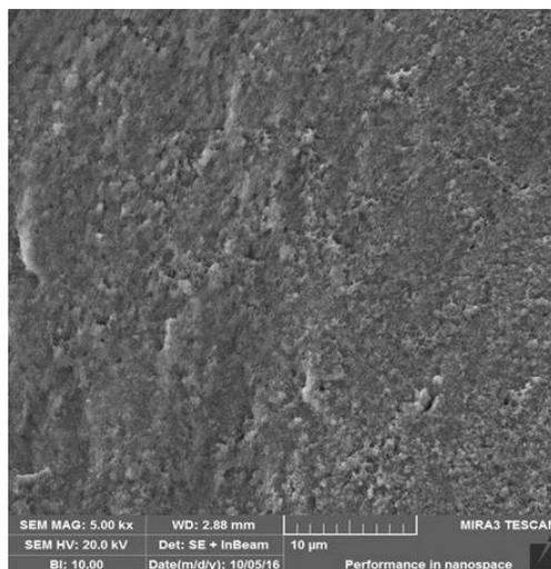
Fig 4: High magnification image of a group A file showing a flatter surface in the peripheral region than the mid region
