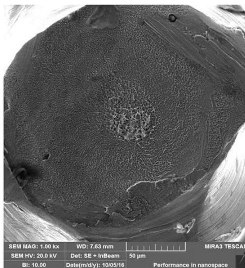
Fig 5: Mid region of a Group B file showing a dimpled surface
