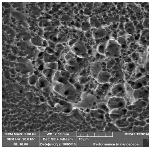
Fig 6: High magnification image of the mid region of Group B file showing dimples
