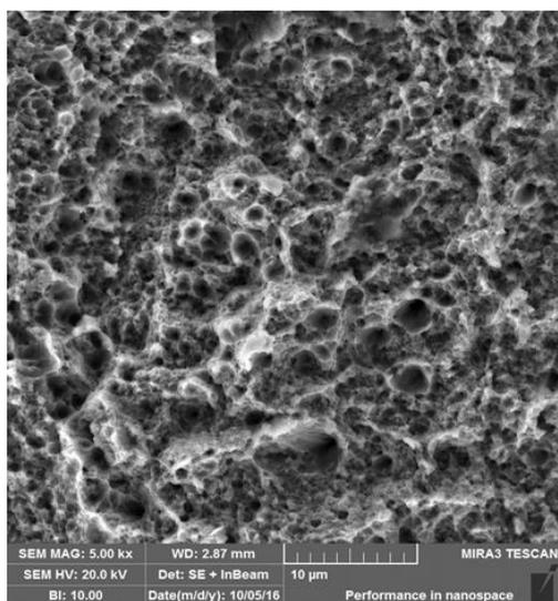
Fig 2: High magnification image of the mid region of Group A file confirming the presence of dimples
