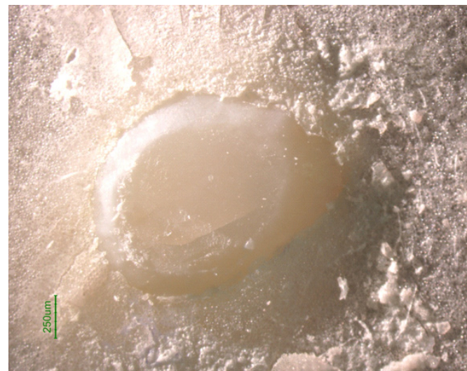
Fig 5: Adhesive failure at enamel-adhesive interface (no composite on enamel)
