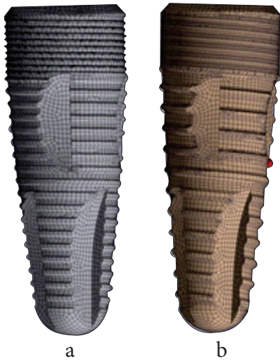
Fig 3: 3.8mm diameter implants with pitch of thread set at 0.4 mm (a) and 0.65 mm (b).
