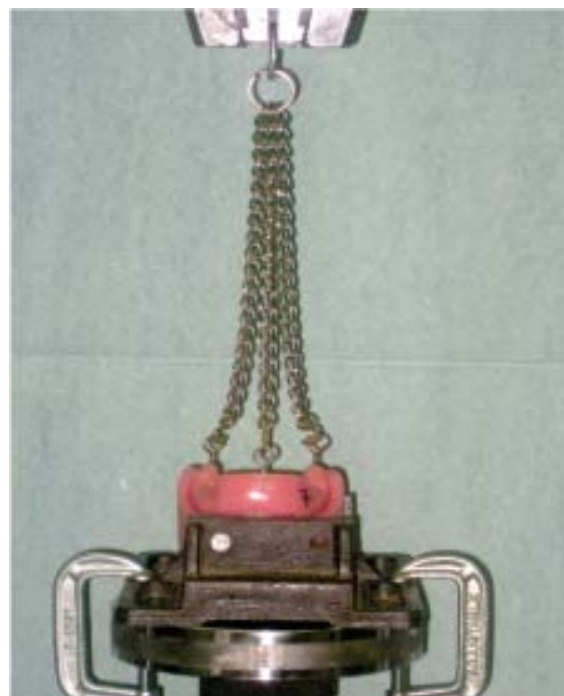
Fig. 3: Position of the chains for the 3-point vertical pull-out which connected to the metallic hook of Instron testing machine.
