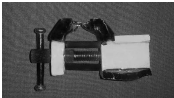
Fig 2: Custom made vise to fracture the tooth
