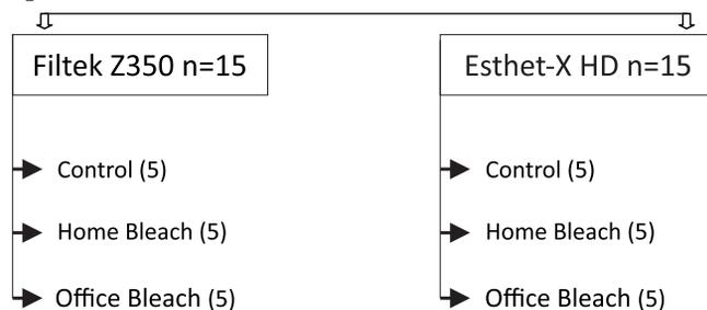
The control group samples were immersed in distilled water for 14 days. Once all samples have subjected to bleaching process, they were again tested for Vickers hardness.
