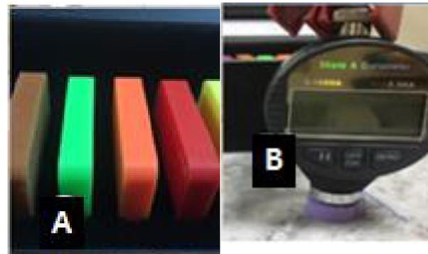
Fig 2: Hardness Testing: A, Standardization blocks of the durometer; B, testing of the alginate samples by the durometer
