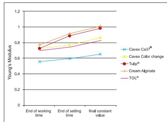
Fig 3: Trends showed by the elastic moduli of the different materials. Significant difference was found between the groups (p<0.05)
