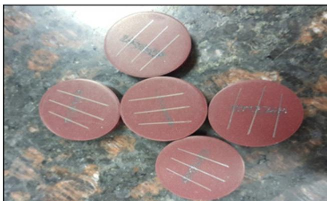
Fig 1: Mounted specimens for microhardness testing
